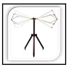
**Internal Choke** An additional feature of the antenna is its highly effective internal choke, which provides immunity to externally induced imbalance.
